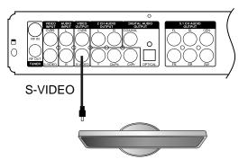
Connect your recorder with the S-Video cable, if the TV has an S-Video input. Do not connect the yellow video cable if you are using the S-Video cable.
